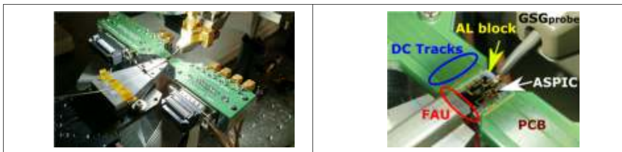
Fig. 1. PIC evaluation platform: application specific (AS) PIC; aluminum block (AL block); Ground-Signal-Ground (GSG) RF probe, fiber array unit (FAU).
